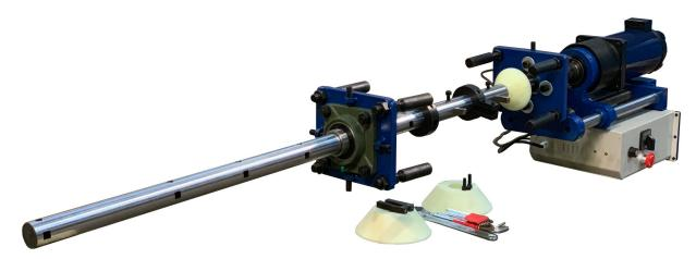
Boring bar size: 40x1500mm, Boring hole diameter: 45-150mm, Stroke: 300mm Max feed depth: 2mm on one side (Clean cut), Main power: 750W. 220V, Feed power: 120W. 220V Speed: 0-100rpm, Power: Brushless AC Motor, Surface roughness: Ra3.2 Processing roundness: ≤0.05mm, Control mode: Electric box panel control
